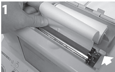
Lever printer locked in print position (down).
